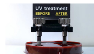
Fig.5 Reaction when the implant is immersed in real blood prior to and after the UV Activation (Source: DIO R&D Institute)
