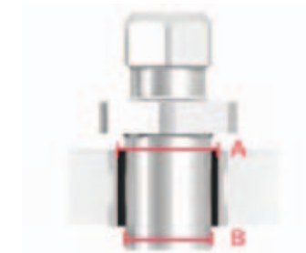
Image 26: Illustrating the difference between the diameters of the implant connector and guiding sleeve
