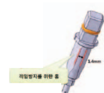
Image 27: Implant connector designed to limit the surface area facing the surgical guide to avoid jamming effect.
